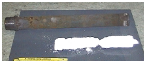
Fig. 3: Precipitate of Na_2SO_4 after an SCWO run
